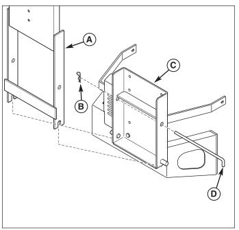
Figure 11. Install Back Plate (Flat Style Bumper shown)
